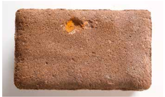
Fig. 12: Paver with lumps of pigment on the surface
