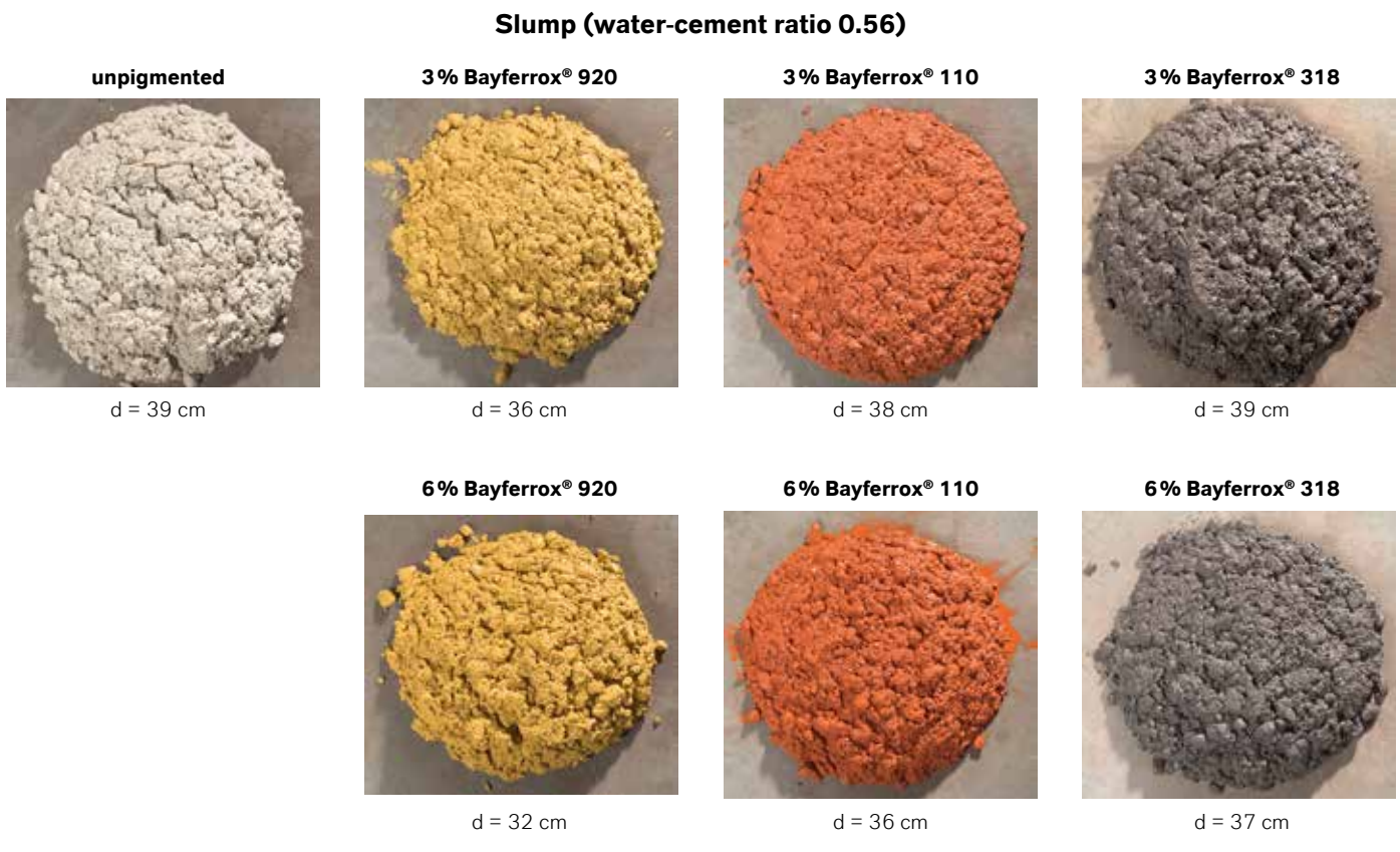
Fig. 20: Slump test comparing unpigmented and pigmented in-situ concrete
