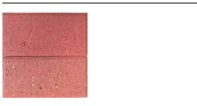
Fig. 17: New and weathered paver, on which the color of the sand is evident
