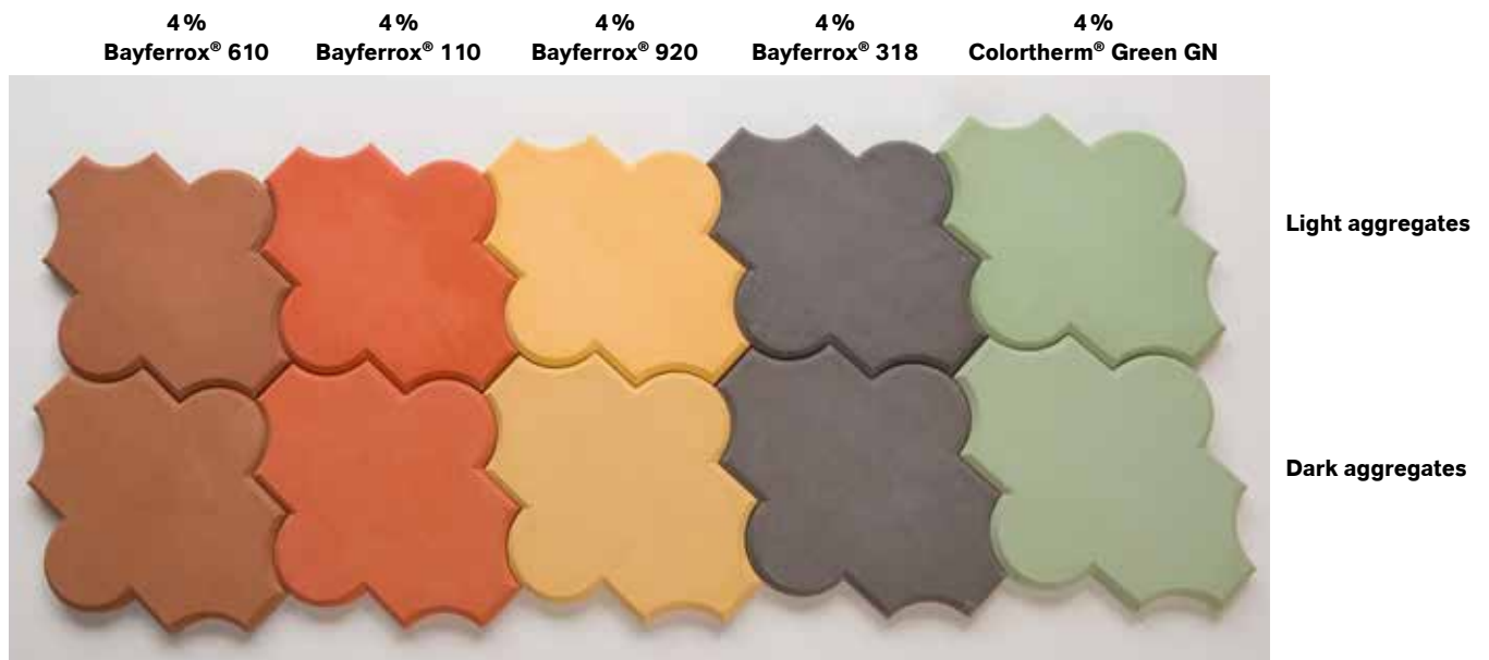
Fig. 7: Influence of the aggregate color on the shade of the concrete
